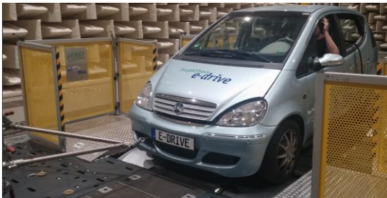
Figure 3.5: Mounting the test vehicle on the roller dynamometer test bench (Alhanouti & Gauterin, 2023b).
