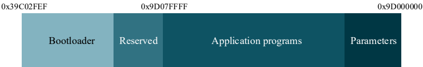
Figure 2.14: Flash memory organization of \mu C-based system, example from Microchip PIC32MZ devices [107].
