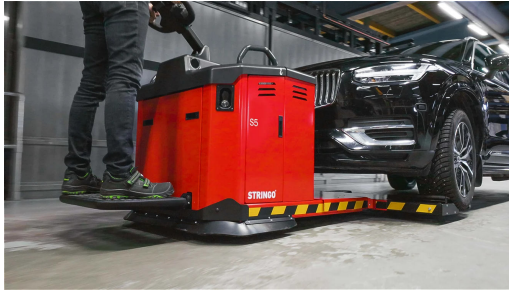
Figure A.1: Vehicle movers used in the automotive end assembly, based on Stringo AB [148]
