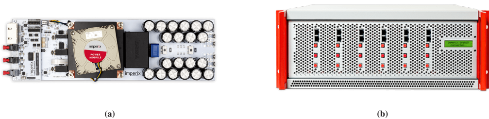
Figure 3.13: The imperix power converter module PEB8038 in (a) with the closed modular rack in (b), courtesy of Imperix [51].
