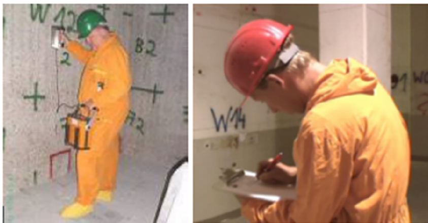
Figure 1: Manual measurement of the interior surfaces of the building and logging of the measurement data (PreussenElektra GmbH 2016).
