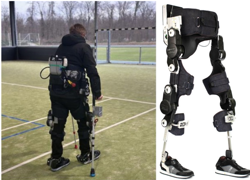
Figure 2. Example of a lower-limb exoskeleton: TWIN exoskeleton. Right image adapted from Semprini et al. (2022).
