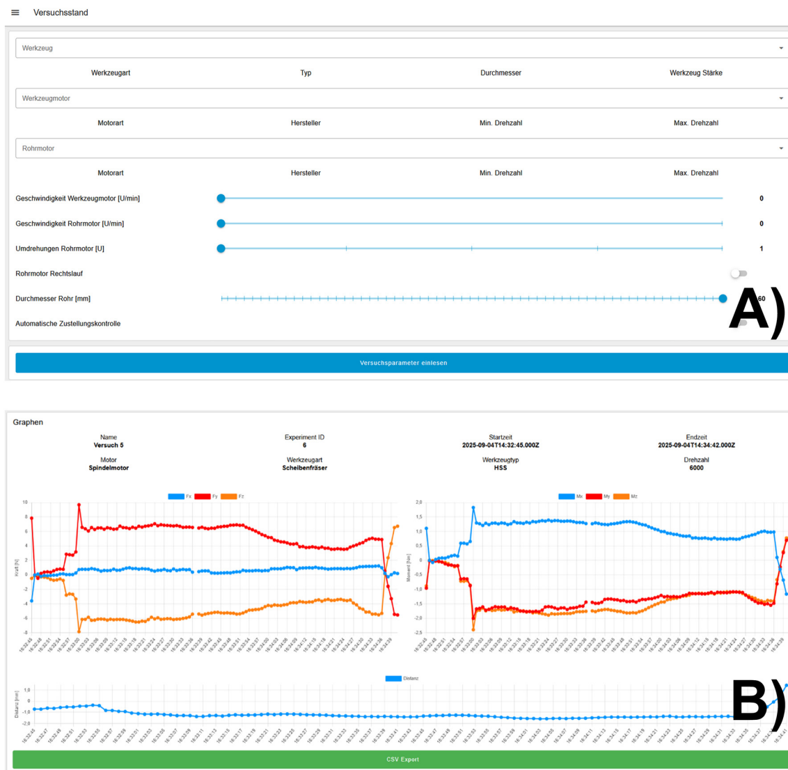
Figure 3: Various dashboards for controlling the test bench (A) and visualizing the recorded data (B), developed with Node-RED.
