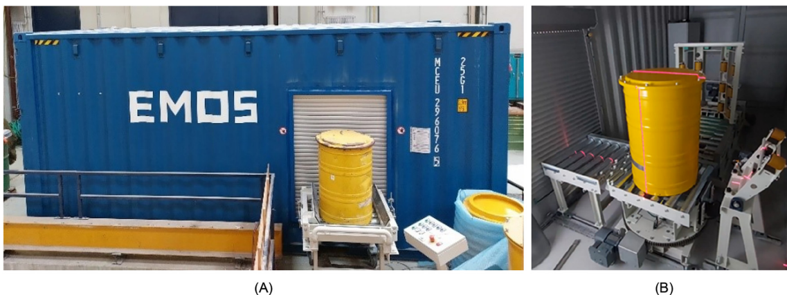
Figure 1: EMOS inspection unit. (A) EMOS container, (B) Turntable with barrel centering device.
