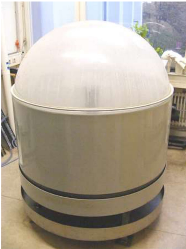
Fig. 2 Salt spray chamber, located in the laboratory of the Institute for Steel, Timber, and Masonry Structures
