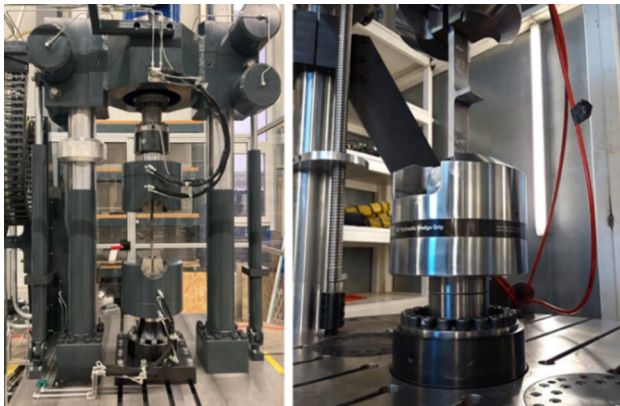
Fig. 10 Servo-hydraulic test rig (left) and resonance test rig (right)
