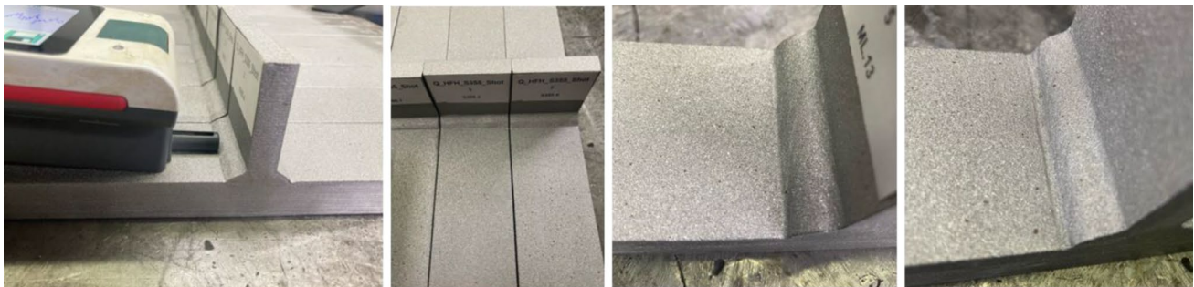
Fig. 7 HFMI-treated specimens of the TS detail after blast cleaning
