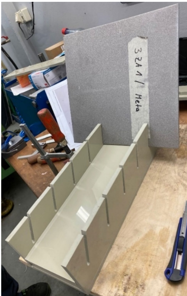
Fig. 4 Polypropylene holder for the small-scale specimens
