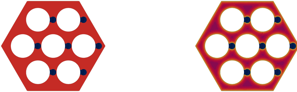
Figure D.11: Uniform (left) and power-law (right) inflow profiles of the seven-pin wire-wrapped rod bundle.
