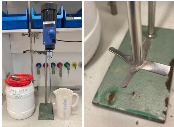
Figure 83: Mixing set-up (left) including the IKA stirrer used for the preparation of cement pastes in this work. The samples were mixed in plastic containers, similar to the one shown in the left picture. The material of the mixing container as well as the container size (volume and aspect ratio) should be kept constant within a measurement series to ensure a constant temperature evolution within the paste. The IKA stirrer is equipped with a 4-blade mixer (right). The used IKA stirrer shows the rotations per minute (rpm) in a display above the rotary control, which is calculated from the applied force.
