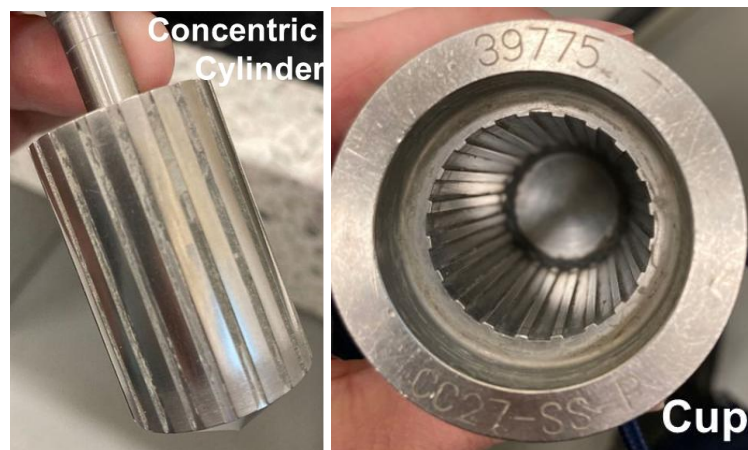
Figure 85: Photo of grooved concentric cylinder and grooved cup. The cylinder has a diameter of 26.6 mm and a length of 50 mm, while the cup has a diameter of 28.9 mm, resulting in a gap of 1.126 mm [222]. This geometry was used with a stress-controlled Anton Paar MCR 302 for all rheometric experiments conducted at Université de Sherbrooke, Sherbrooke, Canada.
