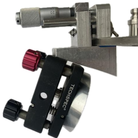
Figure 91: Close up of M2, with additional adjustment screw at the mirror mount attachment to precisely adjust the mirror-crystal distance to the focal length of the off-axis parabolic mirror.
