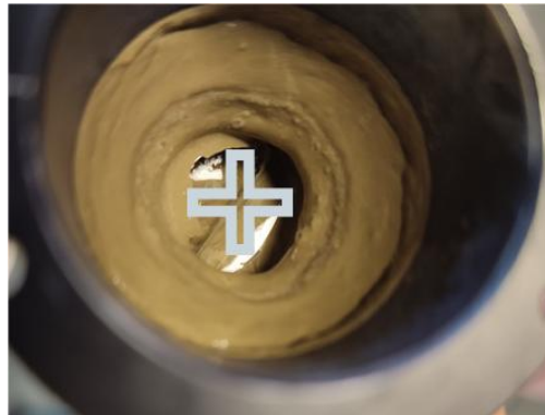
Figure 34: Cement sample after a flow curve was recorded. The grey cross indicates the position of the vane during measurement. The material sticking to the side and the hole at the vane position indicates shear band formation and plug flow. Reproduced from [149].
