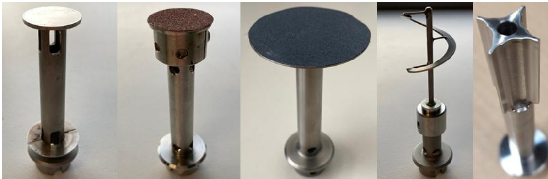
Figure 30: Pictures of different upper geometries tested for the characterization of cementitious materials. From left to right: 25 mm Plate-Plate geometry with smooth surface, 25 mm PP geometry with sandpaper, 50 mm PP with sandpaper, a helix with smooth surface and a four-blade vane with a smooth surface. In the PP configurations the lower geometry matches the upper one. The helix and vane are paired with a Couette (cup) geometry as their counterpart.
