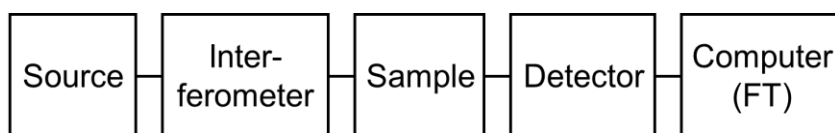
Figure 24: Simplified FTIR instrument, adapted from [141].
