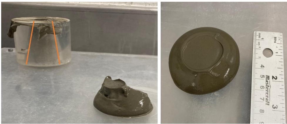
Figure 18: Picture of a spread flow test conducted with a mini cone. In a spread flow test in general, a cone of a defined size is filled completely with cementitious material. As the cone is lifted, the material flows to ideally form a symmetrical, round puddle whose diameter is the so-called spread. The experiment shown on this picture was conducted using a mini cone ( r_1 = 9.5 mm, d_2 = 19 mm, h = 57 mm, V = 37 mL), which in this case was a negative mould inside an acrylic cylinder. The cone inside the cylinder is highlighted with orange lines as guide to the eye. In this experiment, the spread flow test was conducted on a dry acrylic plate in the laboratory of Prof. Ammar Yahia, Sherbrooke, Canada.
