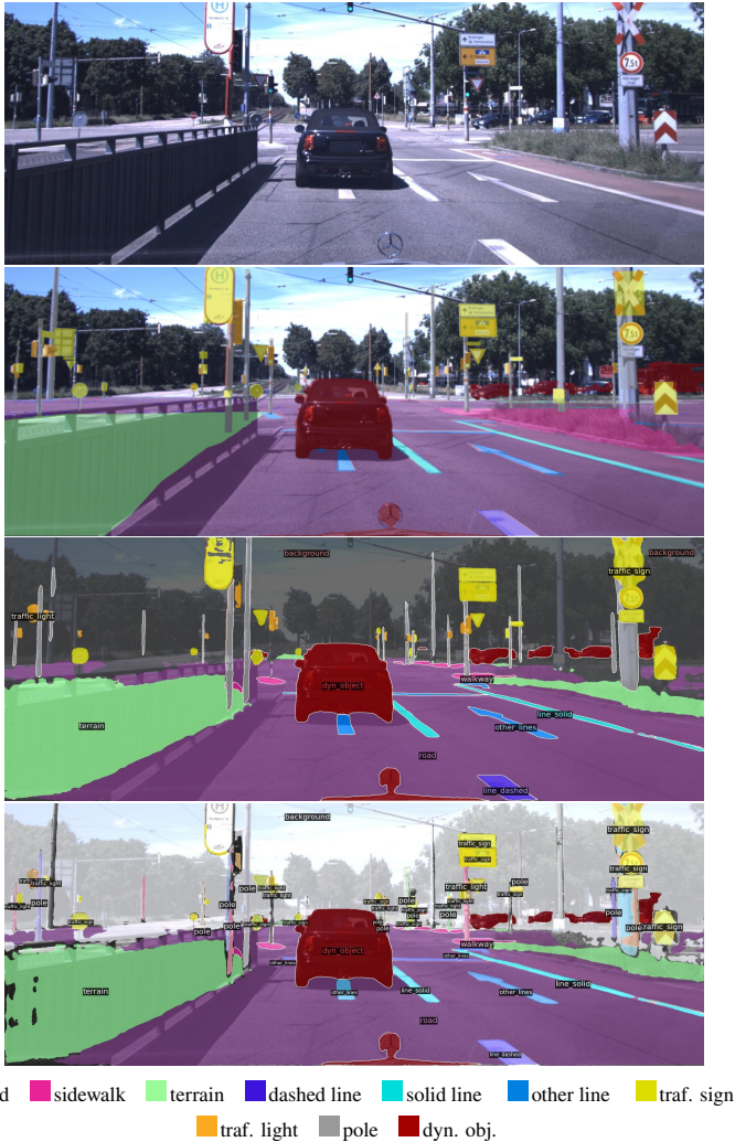
Figure 7.8: Qualitative evaluation of perspective panoptic segmentation. Top to bottom: RGB image, annotated ground truth, prediction results of panoptic segmentation shown as semantic masks and full panoptic output. Examples are from the geographically distinct test set.
