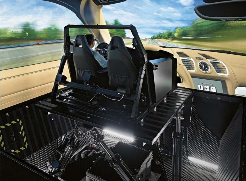
Figure 6.4: Porsche human-in-the-loop driving simulator used in the prototype test group study.
