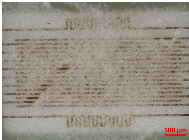
Figure 5.4: SnO 2 NWs on top of IDE array after deposition. Adapted from [2] under CC BY 4.0.
