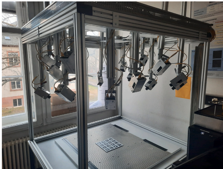
Fig. 7. Extrinsic calibration setup.
