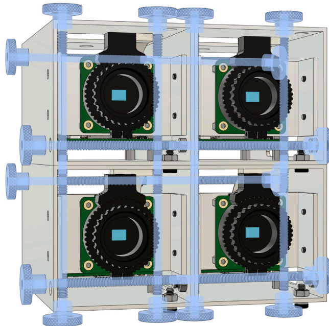
Fig. 3. Stacking of cameras using all-thread and knurled nuts.
