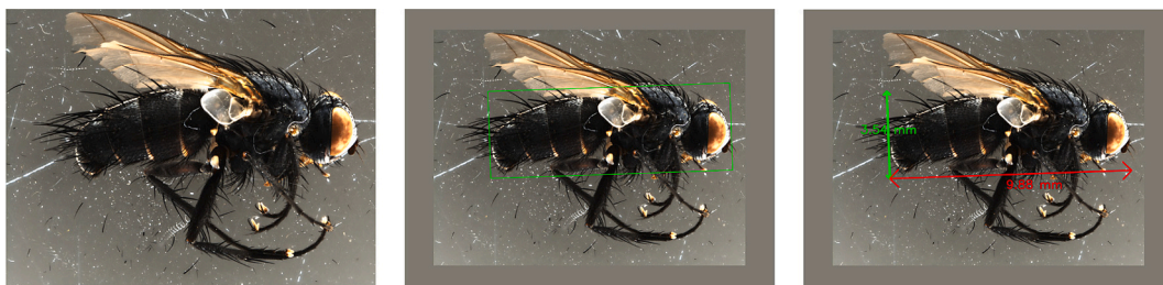
Fig. 2. Workflow of the OBB-based rapid length-estimation module. The input image shows an ethanol-preserved insect imaged individually with the Entomoscope system. Absolute measurements were obtained using setup-specific pixel-to-millimeter calibration factors. Left: input image. Center: predicted oriented bounding box (OBB). Right: final output showing the derived linear length (red) and width (green) measurements. A 10% padded border was used during training to improve OBB placement for specimens near the image edge. (For interpretation of the references to colour in this figure legend, the reader is referred to the web version of this article.)
