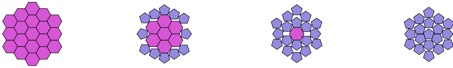
Figure 3.10: Schematic representation of the surface reduction process. The pink hexagons represent iron oxides, and the purple pentagons represent iron. It can be seen that the reduced iron is forced to form domains, as the overall particle size must decrease. For this reason, a fully formed particle with a sufficiently rapid reduction rate will always be porous.
