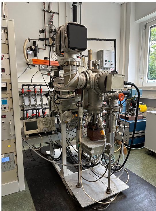
Figure 3.13: Used setup for KEMS measurements at FZ Jülich. KEMS: Knudsen effusion mass spectrometry
