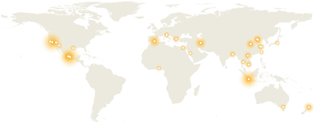
Figure 1: Global extent of land subsidence due to groundwater withdrawal, modified after Gambolati and Teatini (2021). Point halo size is referenced to maximum reported subsidence rates ranging between 1 and 300 mm a -1 .
