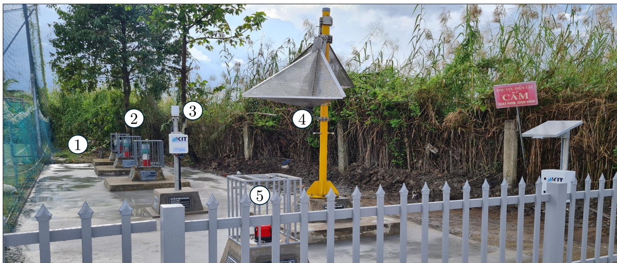
Figure 8: Photograph of the monitoring site GW1, showing the locations of the soil moisture sensor probe ①, three deep groundwater observation wells ②, the meteorological monitoring station ③, the corner reflector ④ and the land subsidence observatory ⑤. Photograph by Felix Dörr, 2022.
