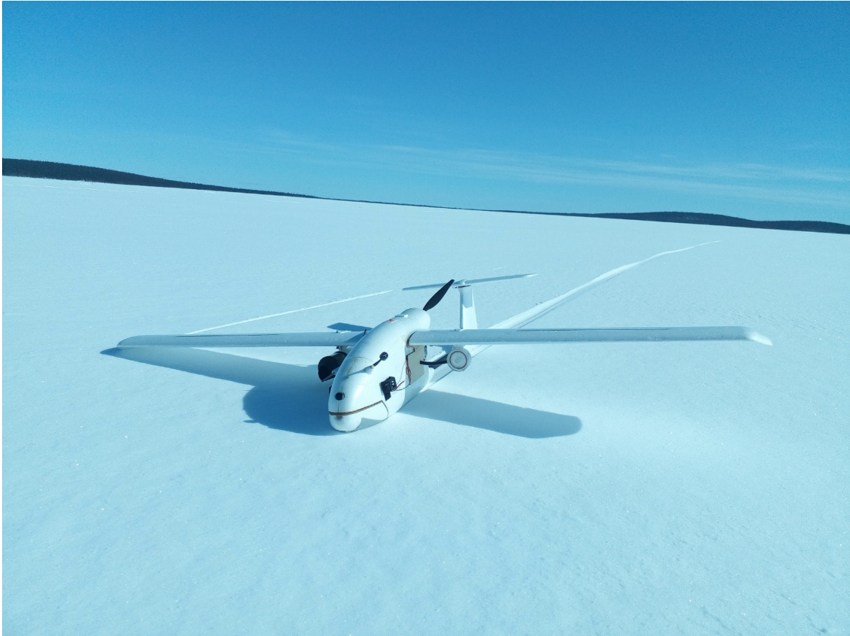
Figure 3.10.: The Skywalker shown with its final setup after a successful flight. The filter holder is visible below the left wing, mounted via the 3D-printed parts shown in figure 3.11. The inlet is blocked until lunch. One of the two ambient sensors is visible on the front left (BME280, Bosch), and the airspeed sensor is visible on the right side (ASPD-7002, Matek Systems).
