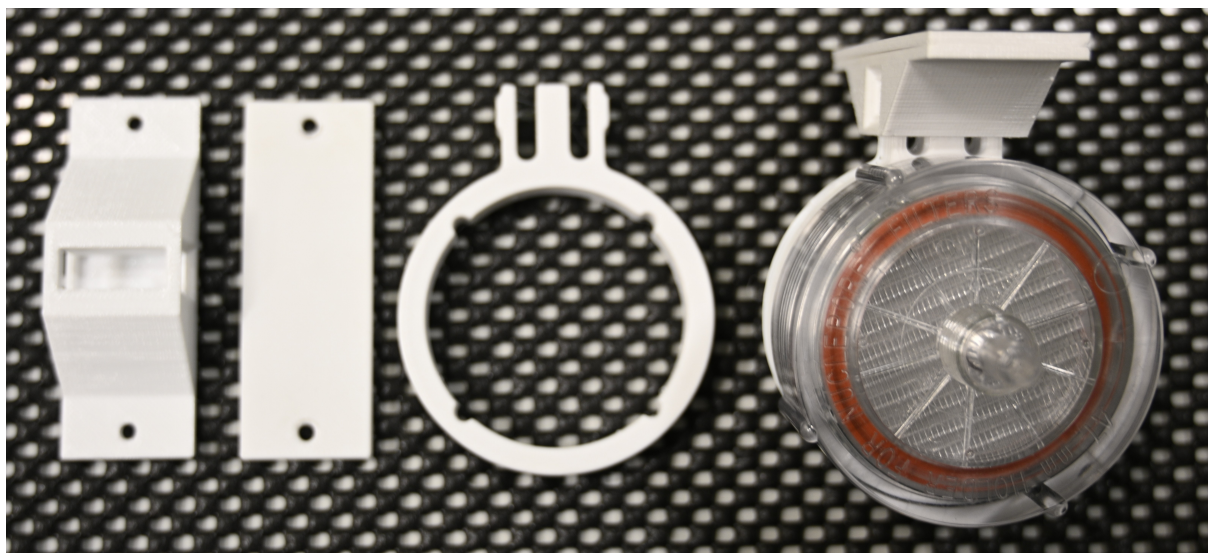
Figure 3.11.: 3D printed parts for mounting the filter holder to the Skywalker wing. From left to right: mount base, mount backplate, filters mount, and final setup. The mount base and mount backplate are fixed to the wing of the airframe. The filter holder mount can be locked onto the filter holder and clipped into the mount base. This allows a quick replacement of the filter holder between flights.
