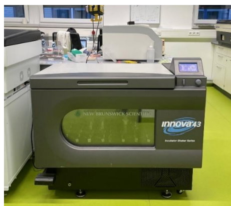
Figure 4.2: The incubator shaker used for static adsorption of GLY/AMPA onto PBSAC.
