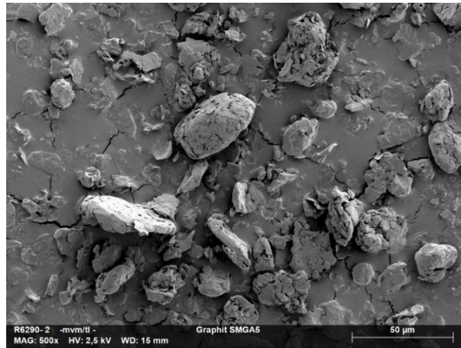
Figure S3.1. SEM image of graphite particles (SMG A5) used as active material.
