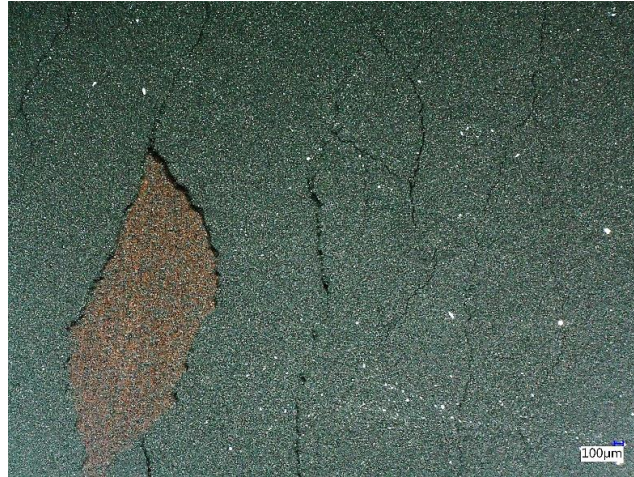
Figure S3.3. Non-calendered 10.1 \text{ mg cm}^{-2} anode with 2.8 % SBR after winding test.
