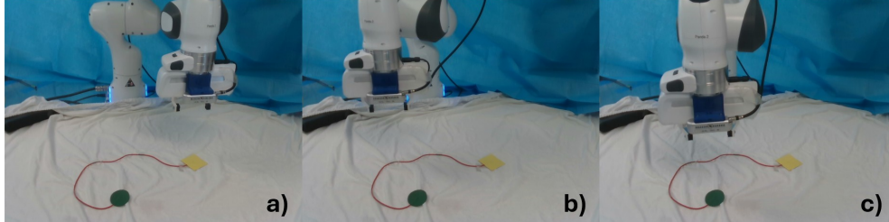
Fig. 3 Feature-following task. From (a) to (c), the images demonstrate different positions along the taken trajectory during the task execution. Starting from a position where the wrist camera is over the yellow marker, the end-effector has to follow the cord until it reaches the green end marker.
