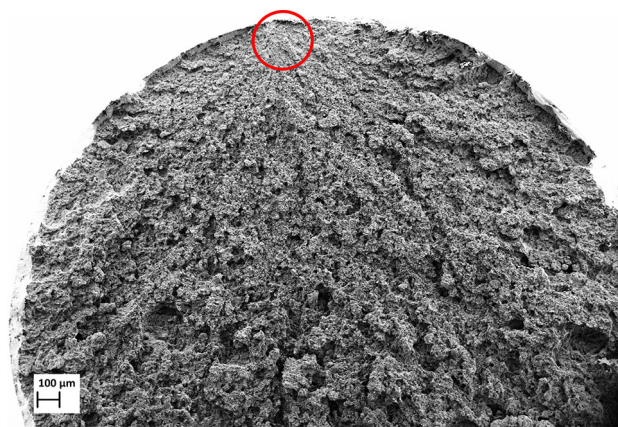
Fig. 23 SEM image of fracture surface of uncharged reference sample with fracture origin indicated by a circle
