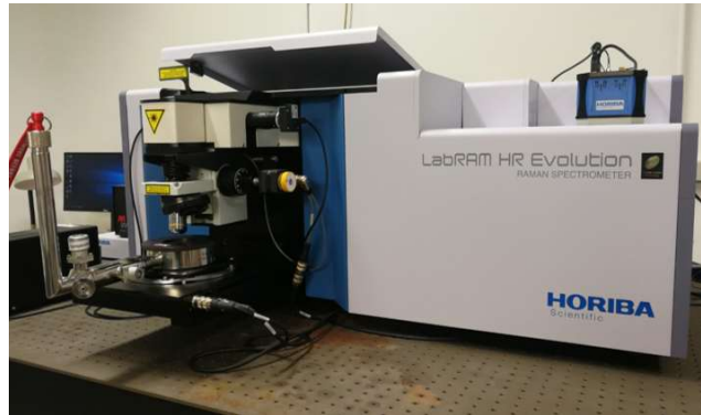
Figure 4.3.: Picture of the Jobin-Yvon LabRam HR Evolution spectrometer used in this study. Figure from [52].
