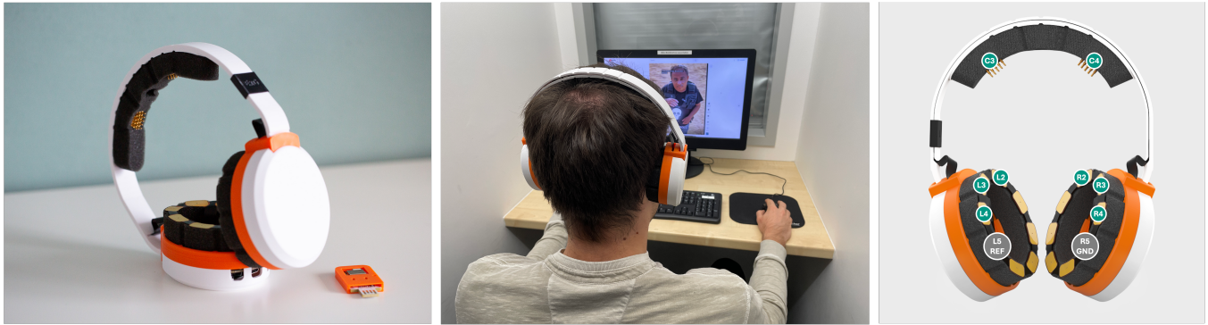
Figure 5: ExG Headphone System (left), in use during the study (center), and schematic electrode layout (right).
