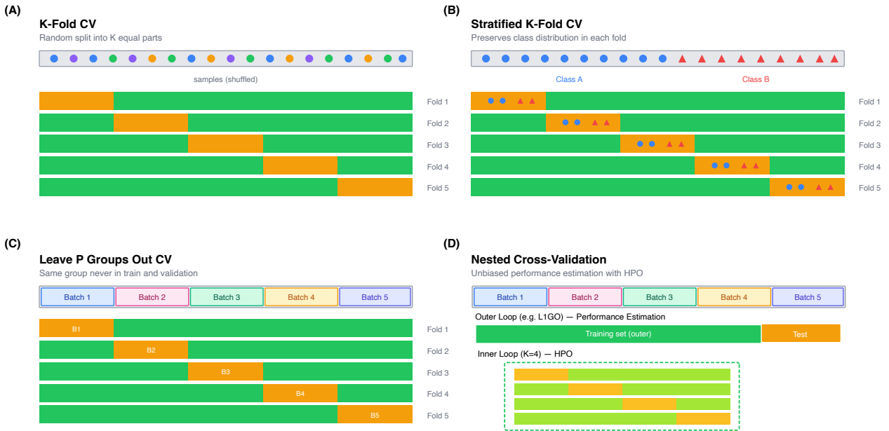
Figure 1.8 Visualization of different cross-validation schemes. (A) K-fold cross-validation partitions the training data into k approximately equal subsets, or folds. The model is trained on k - 1 folds and tested on the remaining fold, with this process repeated k times so that each fold serves as the test set exactly once. (B) Stratified cross-validation extends the basic k-fold approach by ensuring that each fold maintains the same distribution of target variables as the complete training set. (C) When data exhibits a group structure, such as multiple batches from experimental campaigns, group-based cross-validation ensures that all measurements from the same group are assigned to the same fold. (D) Nested cross-validation provides a two-level cross-validation with an outer loop for repeated performance estimation and an inner loop for hyperparameter optimization.
