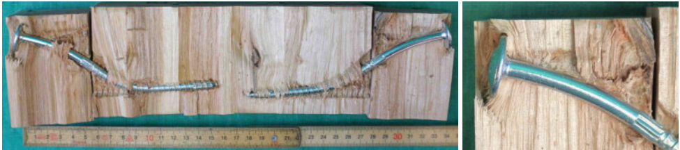
Fig. 3.24: Exemplary head pull-in of non-predrilled screws (type 1) in birch glulam and inclination in side timber at large displacements.
