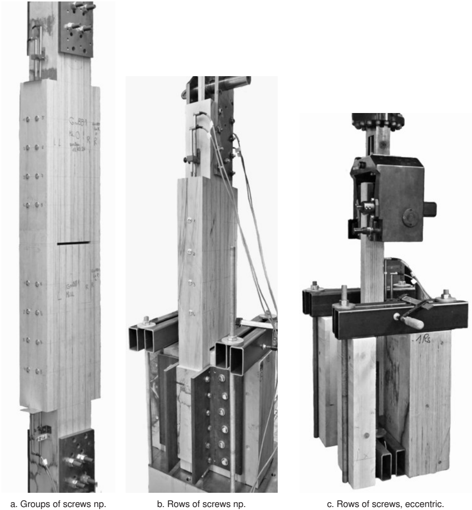
Fig. 3.8: Exemplary images of the test setups for investigated configurations.
