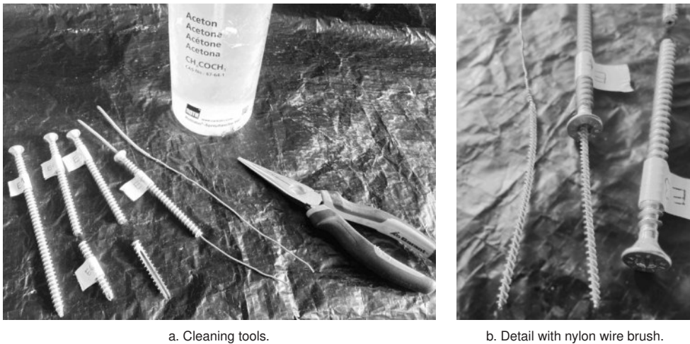
Fig. 4.5: Preparation of boreholes by cleaning.
