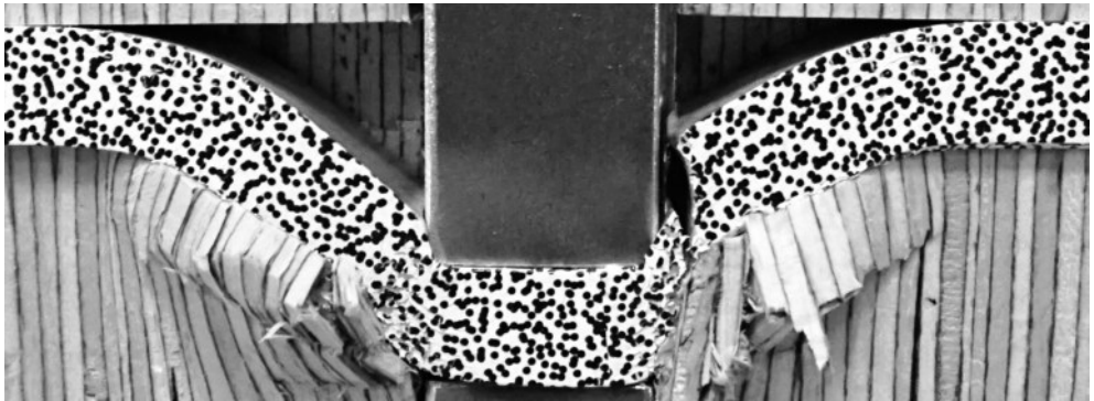
Fig. 5.34: Detail of failure near the shear planes.
