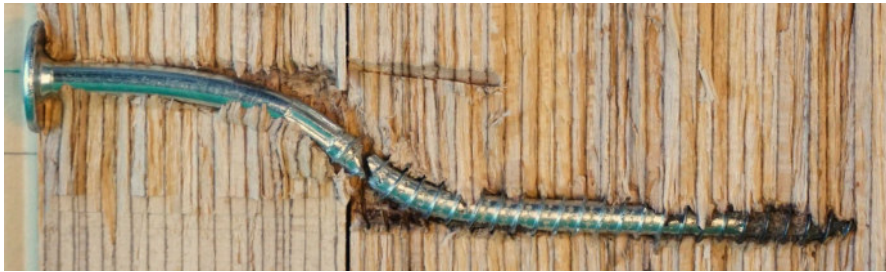
a. Partially threaded screw failed in shear plane with diameter d = 8 mm.
