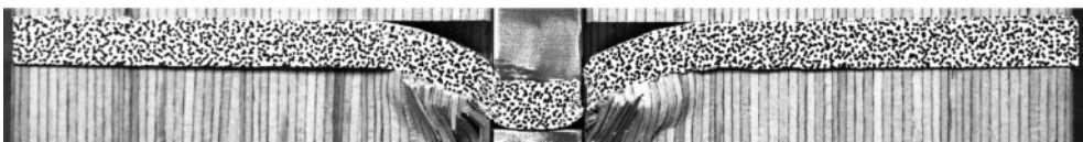
b. Aluminium fastener with head in beech LVL.
