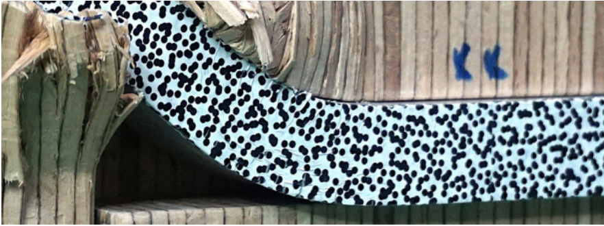
Fig. 6.32: Cracks in the tension zone and wrinkles in the compression zone of an aluminium fastener in beech LVL under large deformations.
