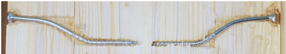
b. Deformation of predrilled screwed connection (type 2).
