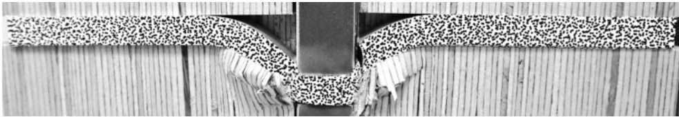
a. Aluminium fastener in beech LVL.
