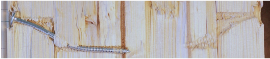
a. Deformation of non-predrilled screwed connection (type 1).
