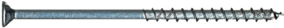
b. Type 2: screw 8x160/80 mm, countersunk head, presunk, predrilled (p) with d_{hole} = 6 mm, shank diameter d_s = 5.8 mm, core diameter d_1 = 5.4 mm.
