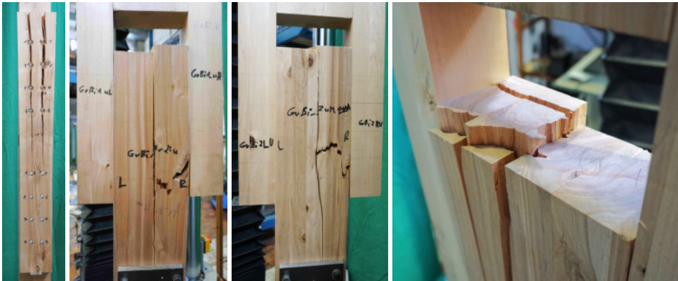
Fig. 3.26: Splitting in grain direction on the left and secondary block shear failure of predrilled screws in birch glulam.
