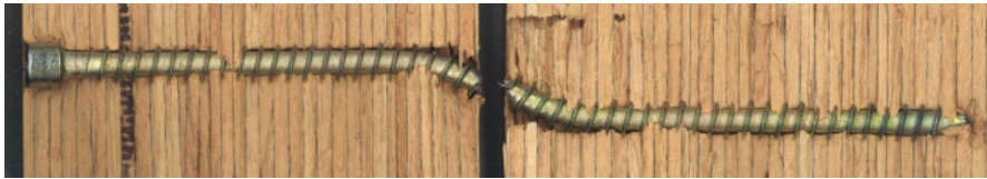
b. Fully threaded screw failed in shear plane with diameter d = 6 mm.
