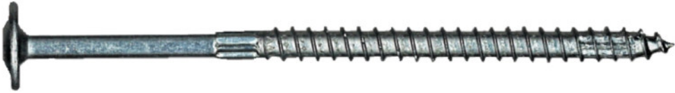
a. Type 1: screw 8x160/100 mm, washer head, non predrilled (np), shank diameter d_s = 6.5 mm, core diameter d_1 = 6.1 mm.
