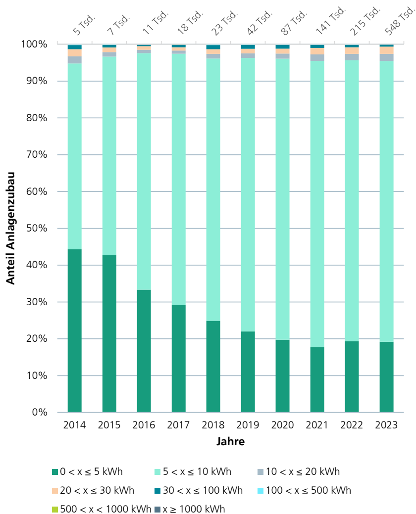
Figure 2.6: Progression of the yearly BESSs installations in Germany, including the distributions over different capacity classes, from 2014 to 2023. "Anteil Anlagenzubau": Share of new plant construction. "Jahre": years. "Tsd.": thousand. Image reproduced from [111].
