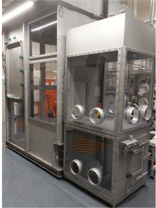
Fig. 13. Glove box, including an in-box crane for heavy parts and a preparation box for dismantling and conditioning.
