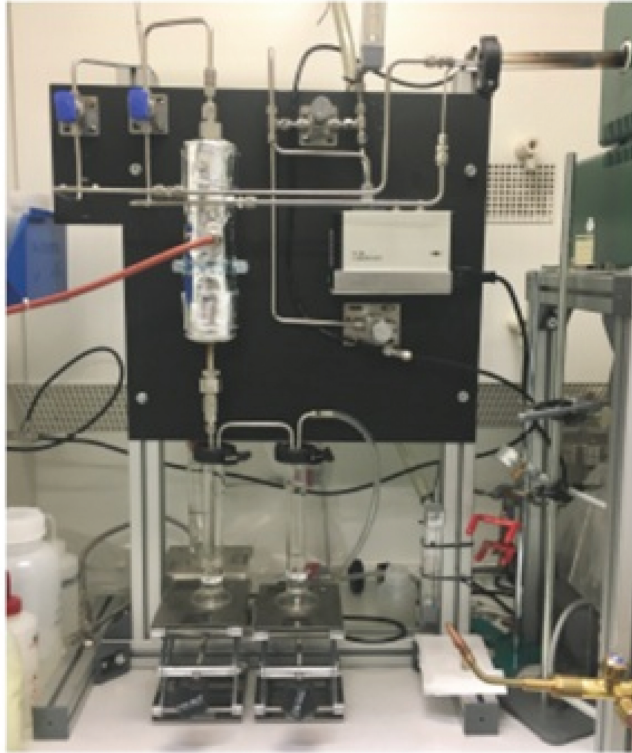
Fig. 11. Picture of the experimental decontamination setup: (left side) analytical part with CuO reactor and bubblers for liquid scintillation grab samples and (right side) oven for the thermal treatment of waste samples.
