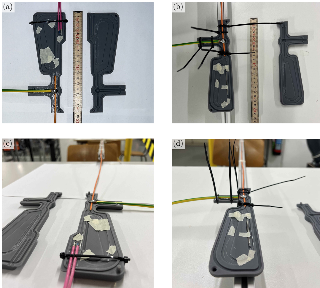
Figure A.2: Photographs of the connector housings of Probe V3 during manufacturing. Both the fiber wiring layout and the soldered electrical connections are presented. (a) and (c) depict the housing, which connects the supply glass-fiber cables and houses two loops of uncovered fiber. (b) and (d) depict the housing containing the fiber splice, which connects both fibers.
