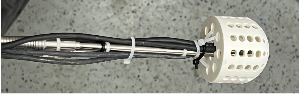
Figure B.5: Photograph of the PT1000 sensors and the PT100 ( Silixa XT DTS) sensors used in a water bath test. All sensors are fixed together with cable ties, and a 3D-printed structure covers the sensor tips to prevent direct contact between the sensor tips and the ice in the ice bath. The black cables of the PT1000 sensors and the long metal tubes of the PT100 sensors are recognizable.
