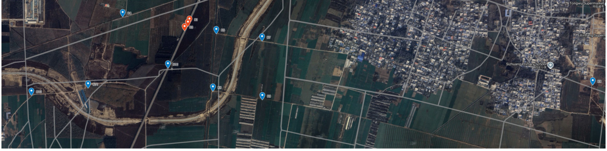
Figure 18. Field HST acquisition geometry showing all twelve seismic stations (R1–R12). Stations R1–R3 (red markers) are the receivers selected for the 2-D FWI because they are approximately aligned with the railway, satisfying the 2-D profile assumption. The remaining stations (R4–R12, blue markers) are distributed in a 3-D configuration around the track and are shown here to clarify the overall deployment. The location of R1–R3 is zoomed in Fig. 19.
