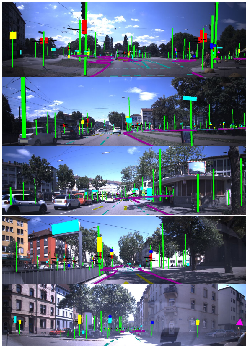
Figure A.9: 2D visualization of exemplar semantic map segment reprojected onto camera image plane of the driving scenario in sequence B10.
