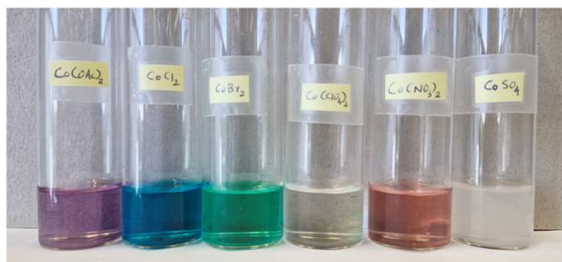
Figure 7.23. The supernatant obtained during the reactions using different \text{Co}^{2+} salts: \text{Co}(\text{OAc})_2 \cdot 4\text{H}_2\text{O} ; \text{CoCl}_2 \cdot 6\text{H}_2\text{O} ; \text{CoBr}_2 ; \text{Co}(\text{ClO}_4)_2 \cdot 6\text{H}_2\text{O} ; \text{Co}(\text{NO}_3)_2 \cdot 6\text{H}_2\text{O} and \text{Co}(\text{SO}_4)_2 \cdot 7\text{H}_2\text{O} .
