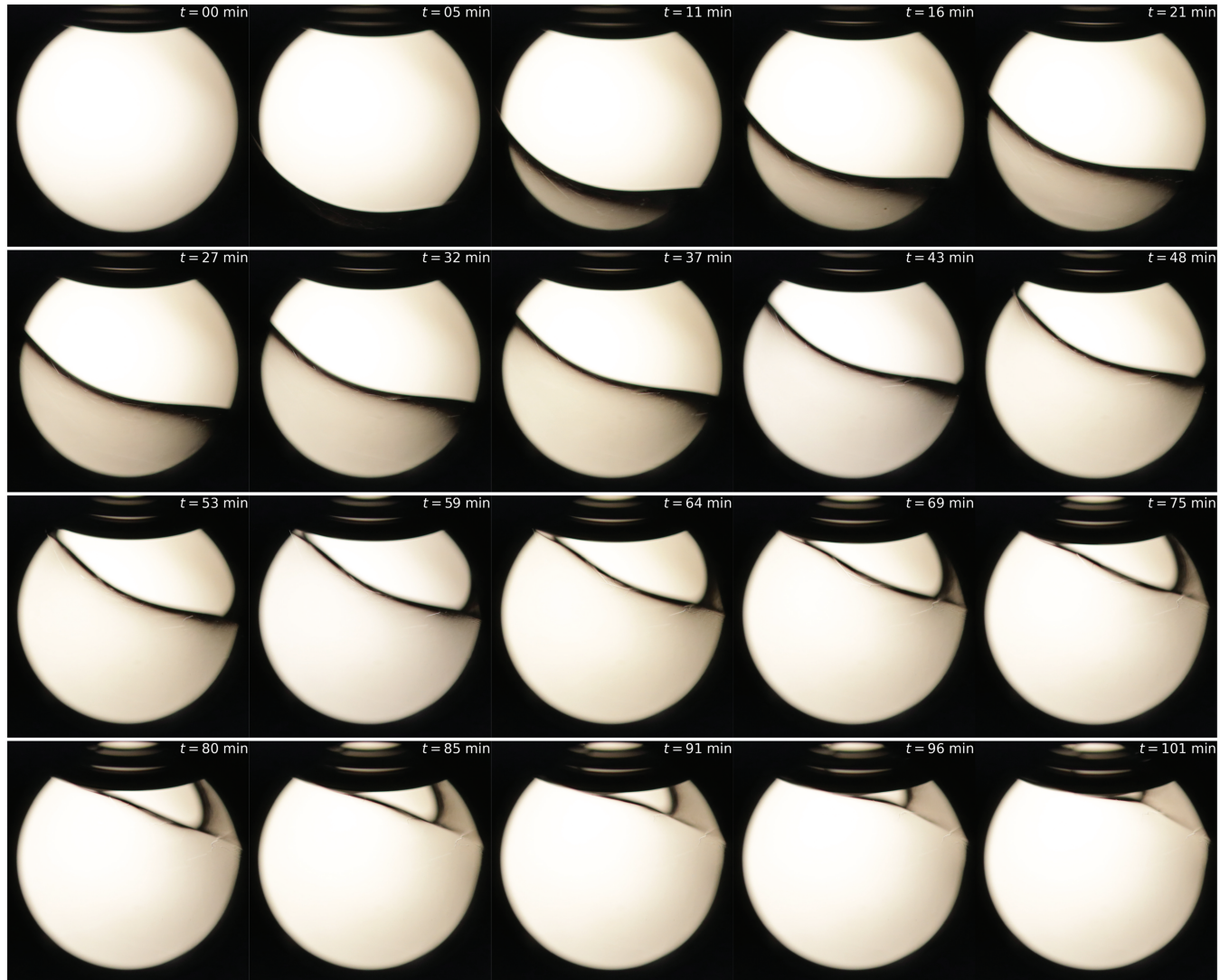
Fig. 3. Slow freezing of liquid H 2 . The cell was approximately 90% filled at the beginning of the shown process. The temperature of the cell during freezing was slightly below \approx 14 K with the pressure gradually decreasing to 0.074 bar. Images are sequentially from left to right, then top to bottom. The entire sequence of images depicts a time span of \approx 100 min.
