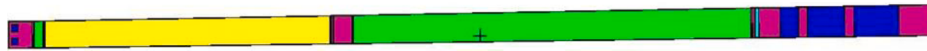
Fig. 4. MCNP model poloidal – radial section of the WLCB BB equatorial outboard slice.
