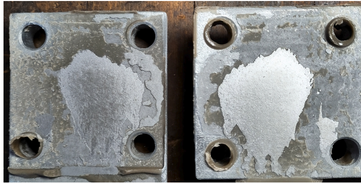
(a) SD-L-15-3: contact surfaces after forcible separation.
