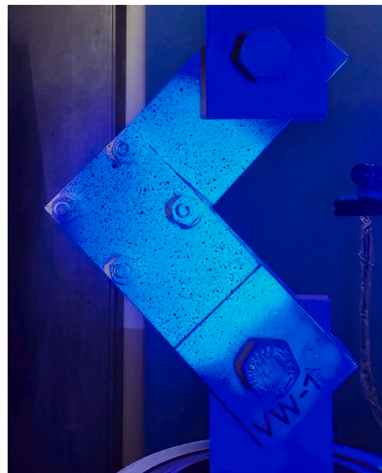
Fig. 6. Representative specimen ready for testing; blue illumination for DIC measurements. (For interpretation of the references to colour in this figure legend, the reader is referred to the web version of this article.)
