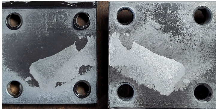
(b) SW-S-15-3: contact surfaces after forcible separation.
