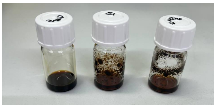
Figure 4.1.13 –Solubility tests of the intermediate (20 mg), with 0.4 mL of solvent (from left to right: Cyrene™, Ethyl acetate, 2-MeTHF, after vortexing for 5 minutes and gently heating).
