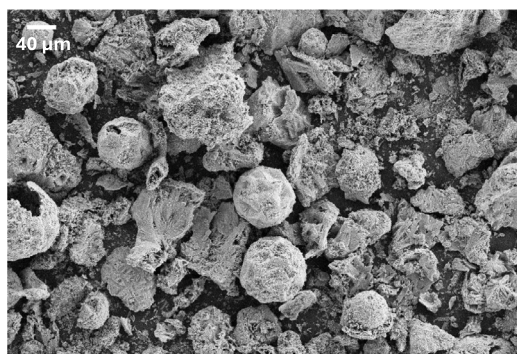
Fig. 3. SEM micrograph of initial \text{Fe}_2\text{O}_3 particles.
