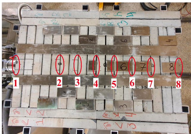
Fig. 5. The HC mock-up from above with the top concrete samples removed. The diagnostic positions are labelled.
