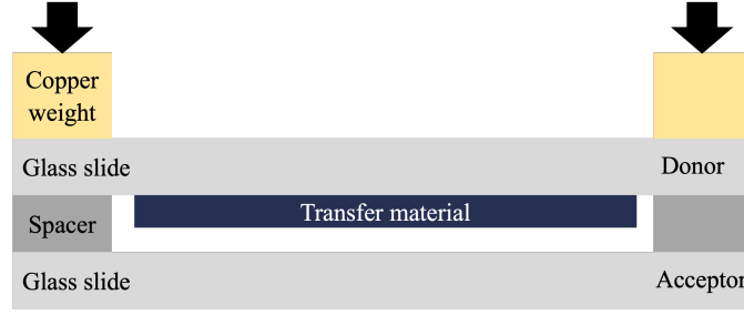
Figure 3.3: Schematic display of the donor and acceptor arrangement for the transfer of liquid pastes.
