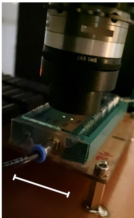
Figure 4.14: Image of an OLED sample being characterized using the MATIS setup. The lens is positioned directly above the sample to capture the emission signal, which is then guided to the spectrometer via an optical fiber. The small yellow dots are emitting OLEDs during measurement. White scale bar = 2.5 cm.
