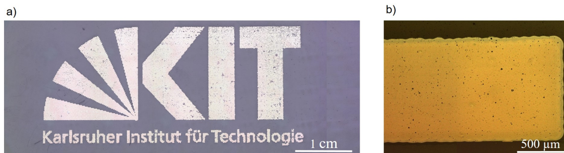
Figure 5.22: Light microscopic images of (a) KIT logo printed with XTPL CL60 silver ink and (b) a continuous area of the same ink printed with a pitch of 100 \mu\text{m} . Color appears different due to different illumination settings.
