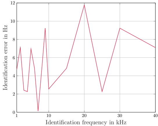
Figure 6.3: Mean of identification error over applied identification frequencies. Identification errors well below the frequency resolution ( \Delta f_D = 82.4 Hz) are achieved for all identification frequencies, preventing tag confusion.
