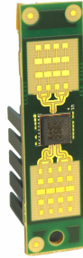
Figure 5.12: mRTS module with mixer chip, antennas, and heat sink on the reverse side.
