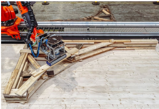
Fig. 5 Case study one ‘frame’, Robotic fabrication process, End effector first generation
