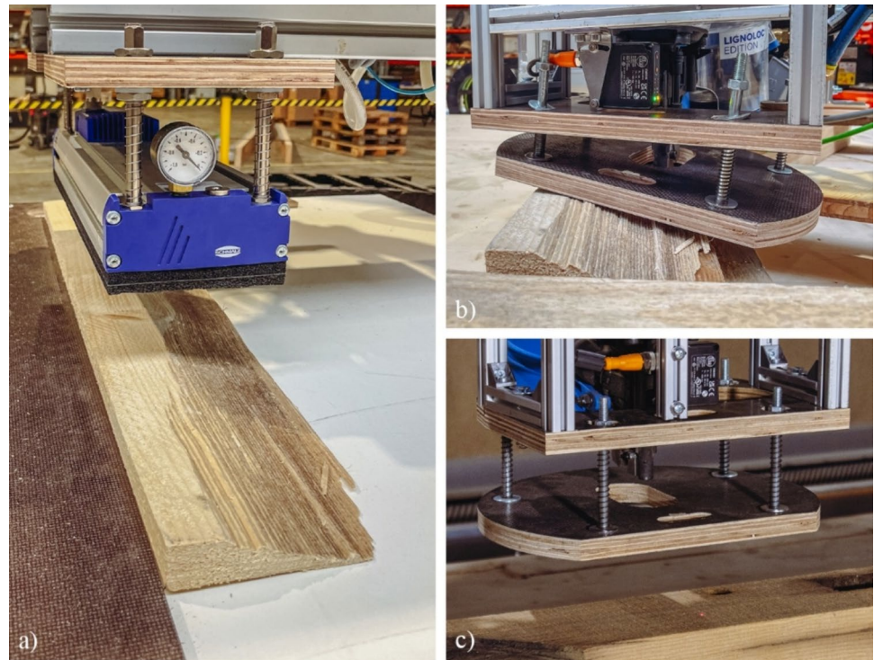
Fig. 2 Spring plungers (a, b, c), Adaptive pressure plate (b, c), Laser distance sensor (b, c)
