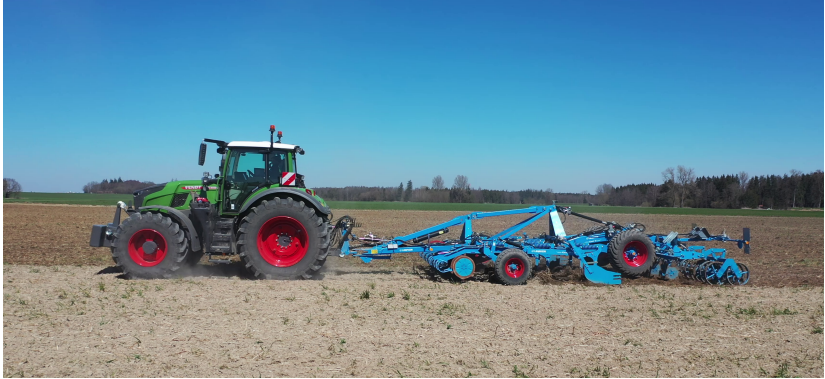
Figure 4.2: Primary combination: Fendt 728 with Lemken Karat 10 KUA.
