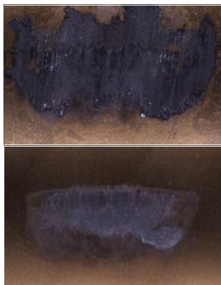
Fig. 6: Resulting profile measurements for cutting fluid one (top) to cutting fluid five (bottom) dependent on time.
