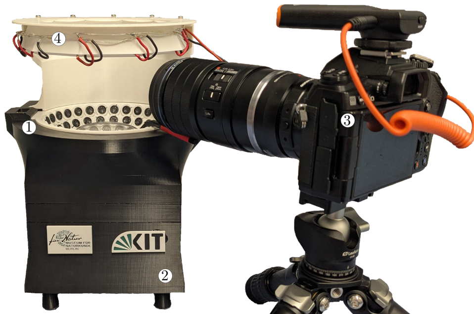
Figure 3: Photogrammetric imaging system using acoustic levitation. The levitator consists of (1) a half sphere with ultrasonic transducers and is controlled by (2) an FPGA with an amplifier board in the base of the setup. For the image acquisition, (3) a macro camera standing on a tripod is used. For a suitable lighting condition (4) a custom made light LED ring with diffusers is used.
