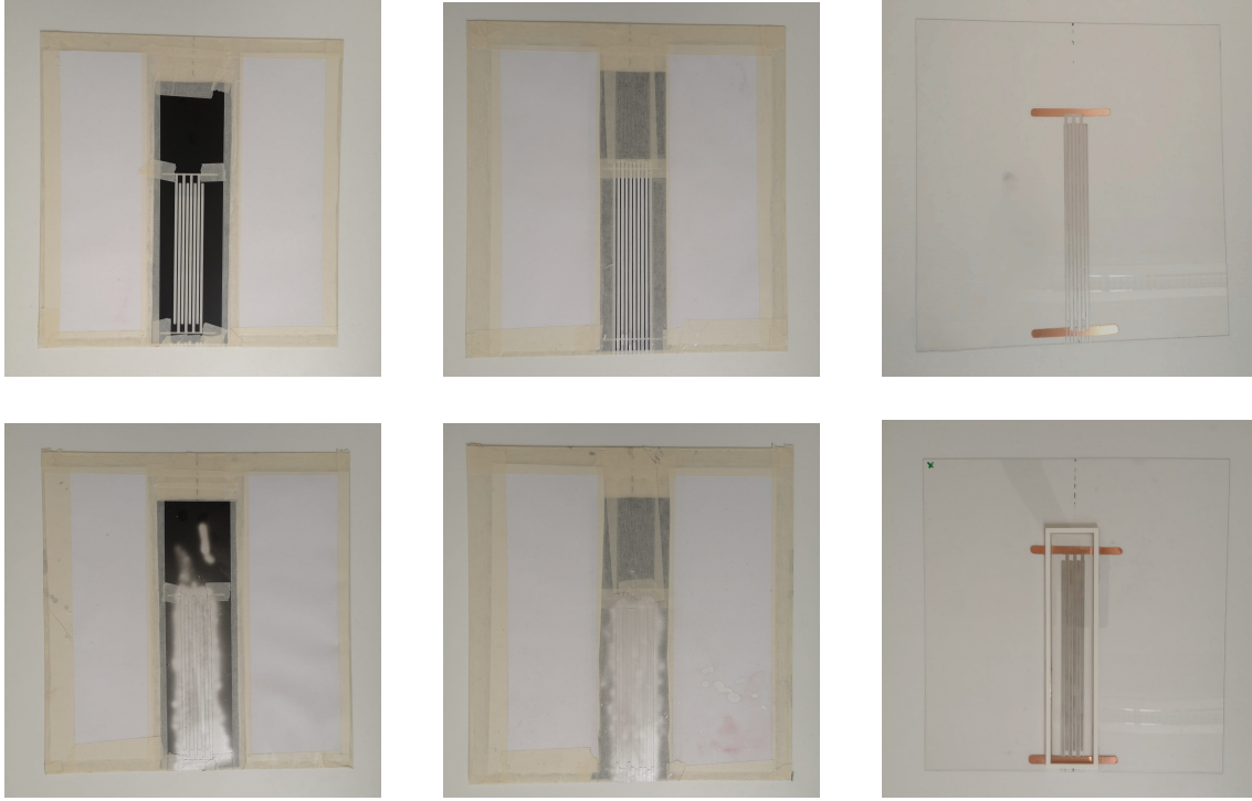
Figure 3.3: PA array fabrication stages. Left: laser-cut stencil on PET foil with lower electrode geometries without and with silver paint. Middle: paper-tape strips as stencil on PET foil with upper electrode geometries without and with silver paint. Right: spray-painted silver electrodes on PET foil with electric connections made from adhesive copper taper without and with 3D-printed frame for epoxy resin.
