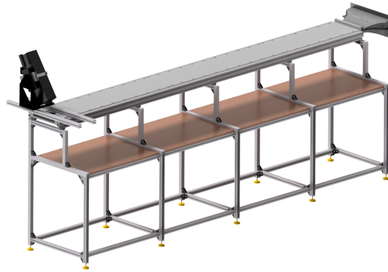
Figure 5.3: Model rendering of channel flow measuring section with LDV-PS measurement setup near the outlet.
