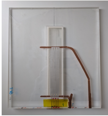
Figure 5.2: PA array integrated in channel wall plate with silver electrodes and copper electrode connections. The wide copper stripes connect the lower electrode groups and the narrow copper stripes the upper two electrode groups to the channel segment front edge.
