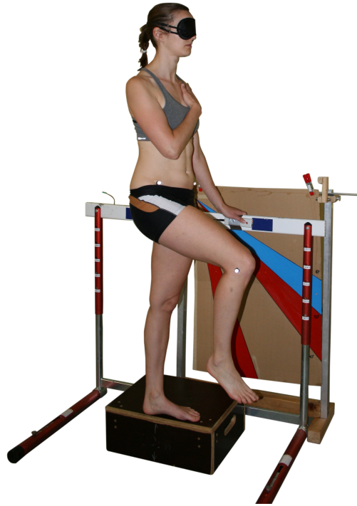
Figure 5.1: Measurement setup for joint position reproduction test. Note. Box height = 20 cm; handlebar with attached switch.
