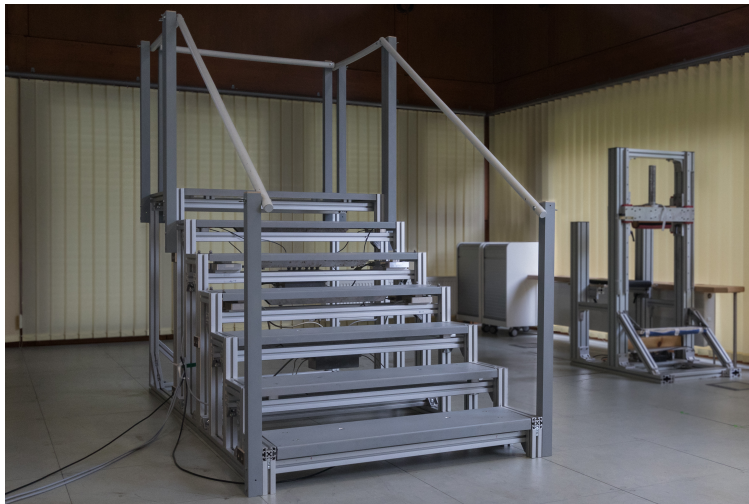
Figure 7.1: Picture of the instrumented staircase. Three-dimensional force plates in steps four and five from the bottom, one-dimensional force plates in steps one to three and six.
