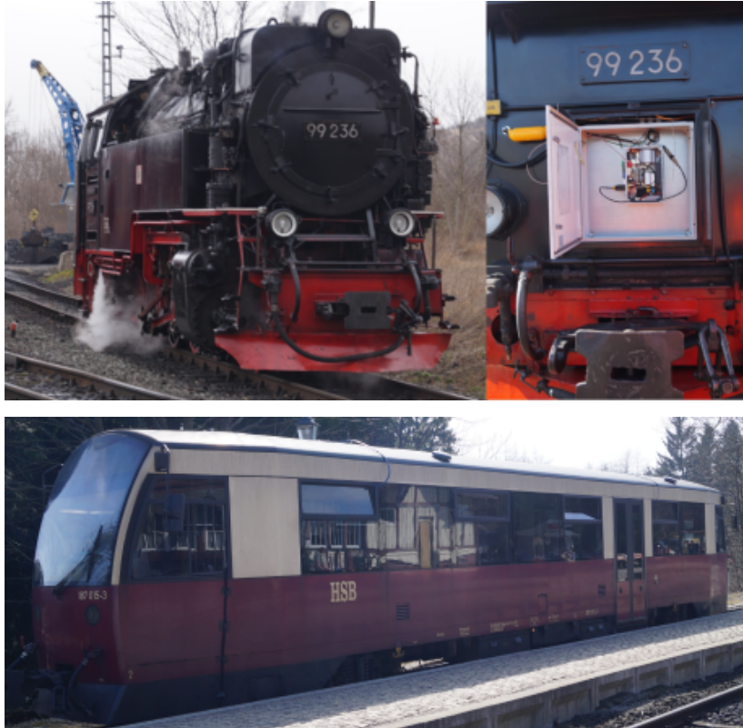
Figure 7.3: (top) Steam engine used during the measurements and steal cabinet on its back with the mounted sensor box. (bottom) HSB diesel railcar. In the railcar the sensor box was mounted directly on the floor inside the cabin.
