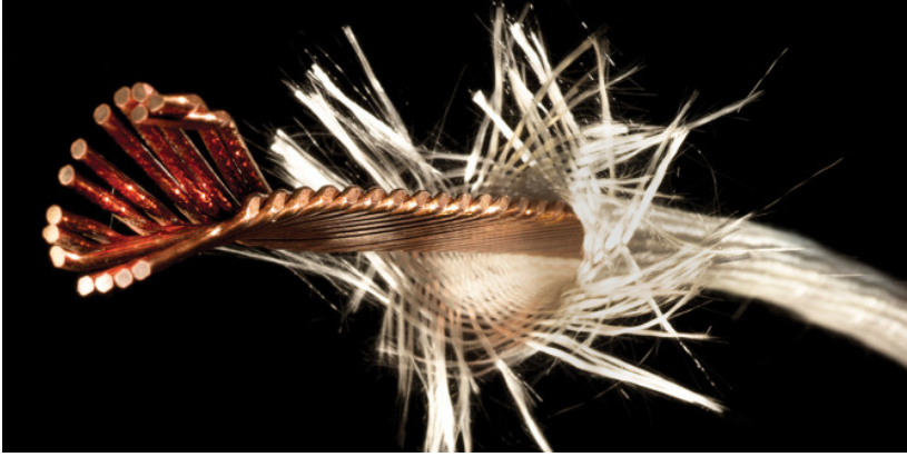
Figure 1.10: Photograph of a Nb 3 Sn Rutherford-type cable with S2-glass insulation [89] . The image exhibits the characteristic flat geometry of the cable with multiple strands arranged in a transposed pattern. The S2-glass insulation provides electrical isolation between turns and creates channels for subsequent epoxy impregnation.
