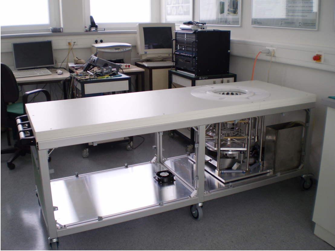
Figure 1.7: 3D USCT II overall structure: (center) the side-cover removed measurement setup; (right, integrated in patient bed) assembled measurement container with sockets for transducers and the rotation/lift mechanics below; (top-left) control PC; (top-right) data acquisition (DAQ) hardware.
