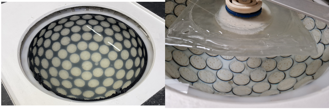
Figure 7.20: (Left), Experiment 2710, water measurement with TAS caps and absorption mats. (Right), another absorption experimental setup with a CIRS phantom.
